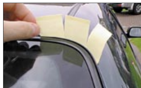
TM27 TrimFast's rigid plastic edge and perforation makes masking windshield, side light and back glass moldings quick and easy.
